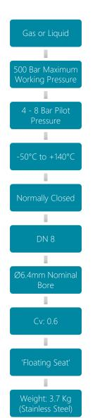
The PSV8 is both compact and robust in construction. High spring force, and a pressure biased valve maximise sealing force, whilst the 'floating seat' ensures optimised concentricity between mating parts.
